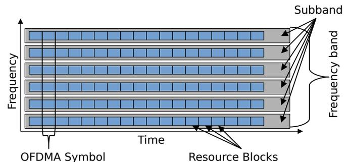
Fig. 5. OFDMA Symbols with frequency and time domain usage with Subbands and Resource Blocks
