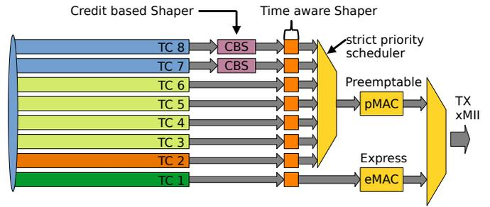
Fig. 9. Egress processing of Ethernet switch port, cf. [13]
