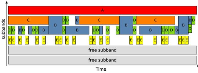
Fig. 8. Frequency assignment to different types of datastreams
