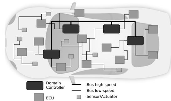
Fig. 1. Domain controller based communication system
