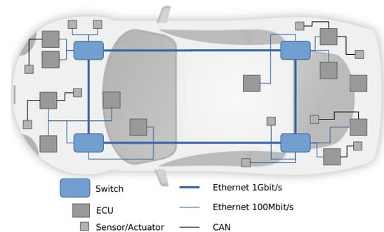
Fig. 2. Zonal backbone communication system
