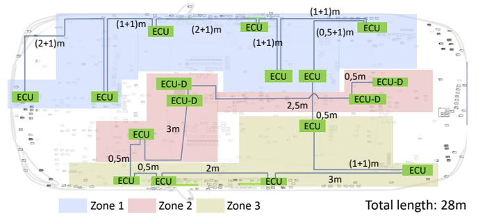
Fig. 7. OFDMA-based Ethernet backbone with cable length
