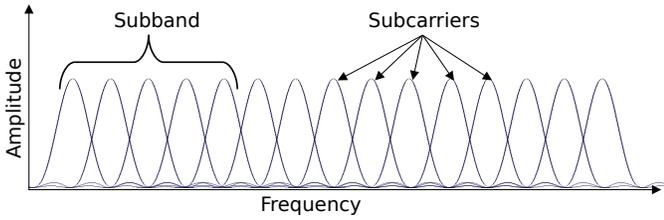
Fig. 3. Correlation between frequency and subcarriers with subbands
