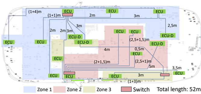
Fig. 6. Ethernet-based backbone with cable length
