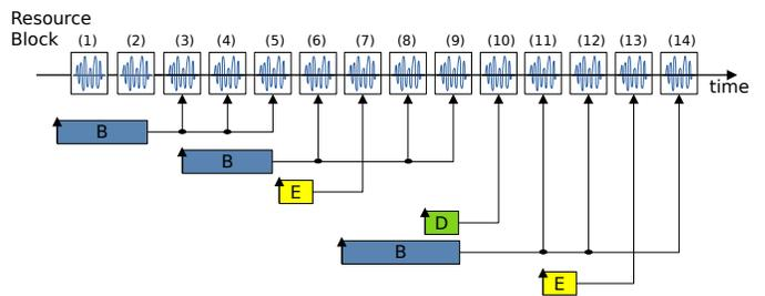
Fig. 10. Assignment of data classes to OFDMA Symbols including preemption for one Subband
