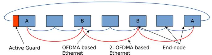
Fig. 13. Redundancy concepts with OFDMA-based Ethernet; either a second cable or a with a active guard
