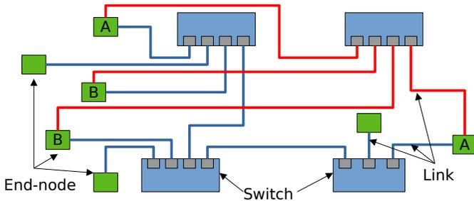
Fig. 12. Redundancy within Ethernet realized with a additional switch and four cables (red)
