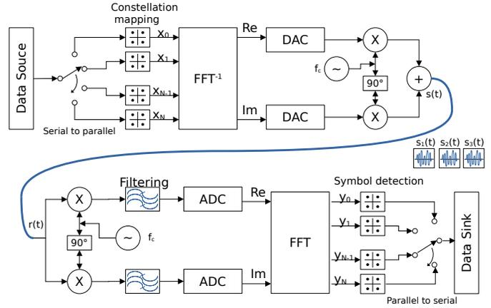
Fig. 4. OFDMA basic function block diagram with IFFT and FFT
